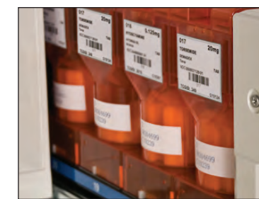
Multiple canisters can be assigned to a single medication to reduce replenishment time. Features bar code verification of right meds and smart pinning to ensure right location.
